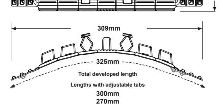
The flexible tabs at the ends of the union can be folded back or trimmed off in order to suit shorter ridge & hip tile lengths
