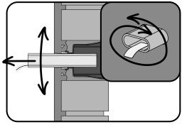
8. Before the render has fully dried and is still in a semi malleable state, rotate the render bung in a soft circular motion to create a slight release angle within the render, allowing it to be gently pulled free. Any rough edges to the hole should be smoothed over once the render is dry.
