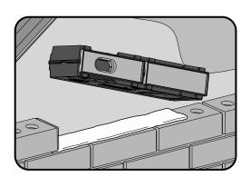
2. Lay a small bed of mortar along the course directly below where the swift brick will sit and against the perp end of the adjacent brick.
