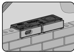
**3.** Bed the product into position, ensuring that the front edges of the brick slips are flush to the brickwork. The product should push down fully onto the brickwork below.
