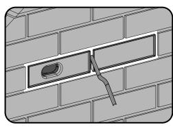
**5.** Once fully built into the wall, the two external brick slips can then be pointed into the surrounding brickwork to finish off the detail.
