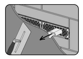
7. Prior to application of the render, partially pull out the render bung using the tab provided to act as a former for the entrance hole. The wall can now be rendered, ensuring that the render is pressed firmly into the open slip holes and evenly around the around the bung.
