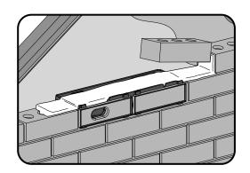
**4.** Continue bricklaying as normal, when laying the course above the swift brick, a small bed of mortar should be laid onto the upper surface. The bricks above will fully bed down onto the top of the product.
