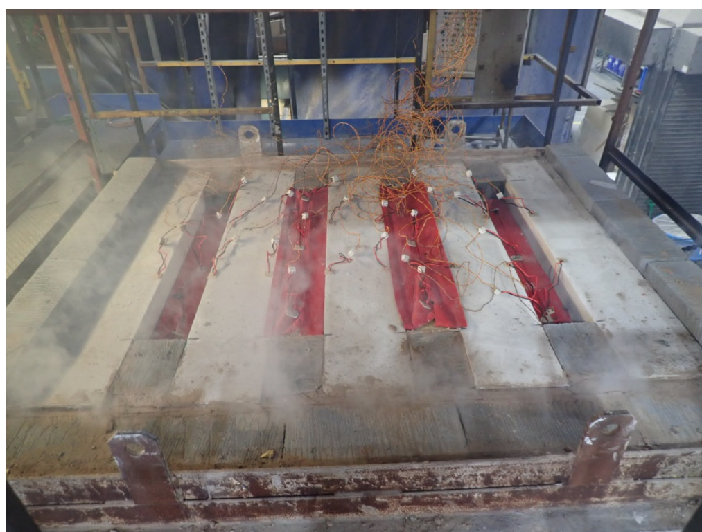
The unexposed face of the floor assembly after a test duration of 30 minutes
