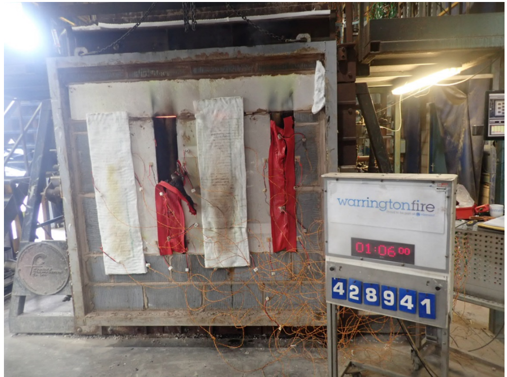
The unexposed face of the wall assembly after a test duration of 66 minutes
